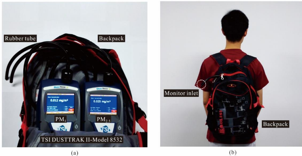
Figure 3. The monitor backpack: (a) the monitor instruments, and (b) the monitor inlet.
