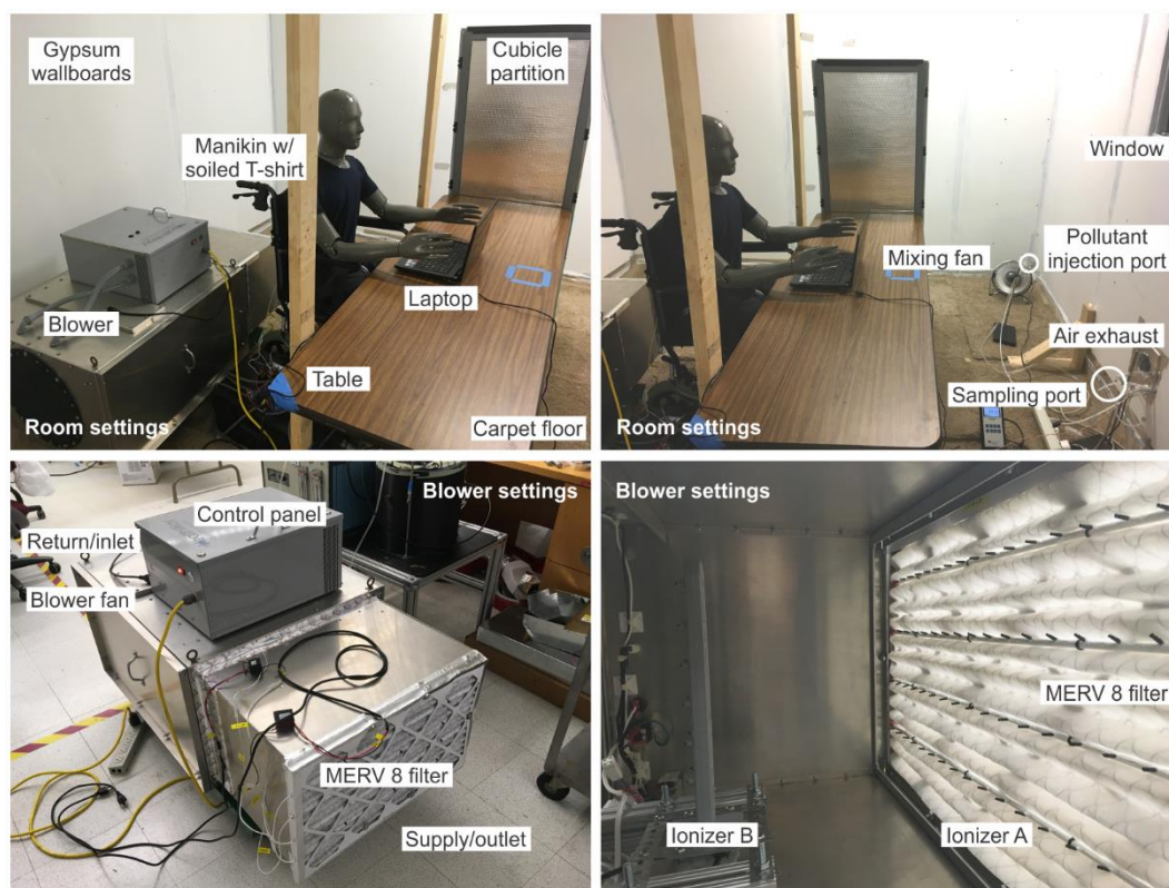
Figure 1. Chamber testing configurations and blower settings.
